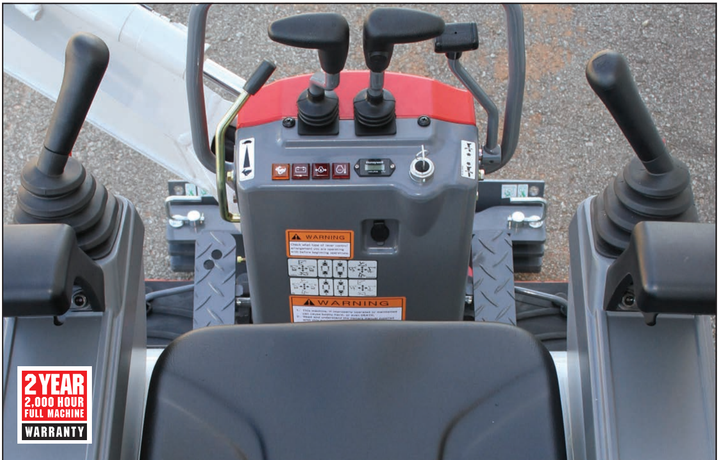
Spacious Operator's Station with New Pilot Operated Joysticks
