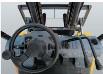
Finger-tip operation with the electric F/R lever
