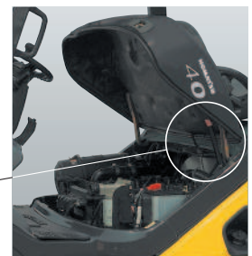
Locking engine hood provides protection while servicing
