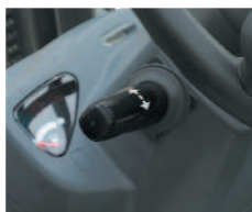
Finger-tip operation with the electric F/R lever
